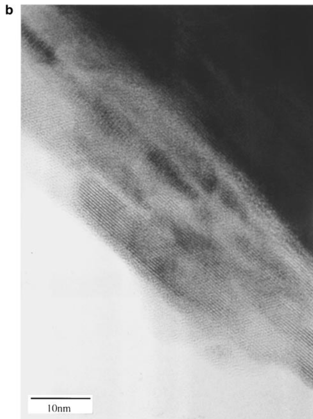
FIG. 5. Typical plan (a) and edge-on (b) views electron micrographs of a (\text{VO})_2\text{P}_2\text{O}_7 platelet exposed to oxidizing reaction conditions.
